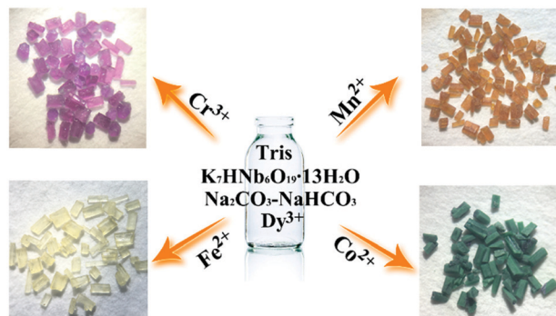
Fig. 1 Crystals morphology of 1-TM-Dy under an optical microscope and the schematic synthesis process of them.
